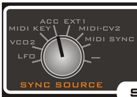
The sequencer can be clocked from seven different sources;
