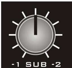
Left; changes the level of VCO1 Sub, which is one octave down from VCO1.
