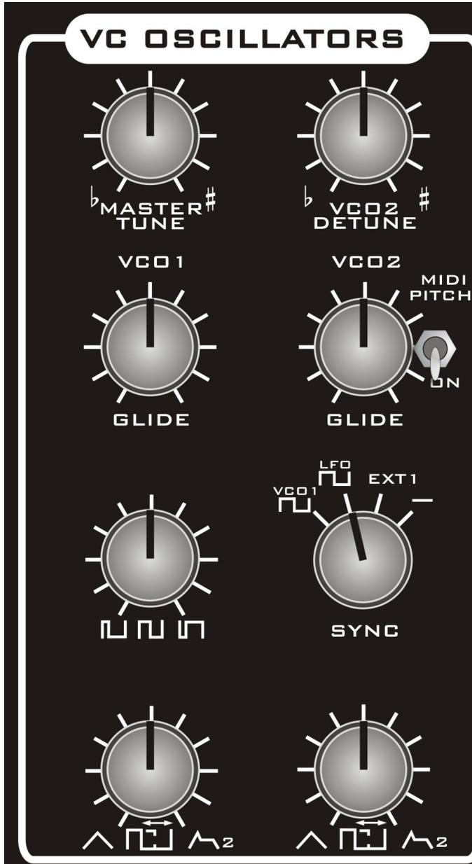
The two VCOs are almost identical, but VCO1 has a manual pulse width control, and VCO2 has a Sync feature.
