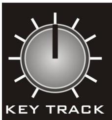
This control routes pitch CV to the filter cutoff. When it is turned up, as you play higher up the keyboard, the filter will open up. This makes the sound get brighter as you play up the keyboard.
