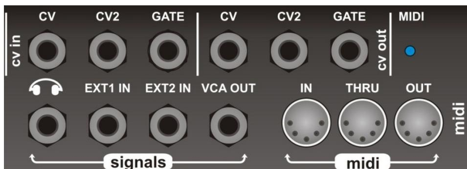
**CV IN:** This is a pitch CV input socket if you want to control the synth's pitch from an external synth. Scaling is 1v/Oct.
