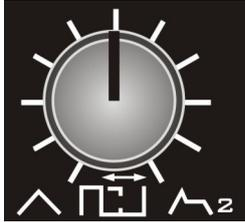
This allows modulation of the Pulse Width of the square wave. It can be modulated by the LFO Triangle wave when turned left, or, by Envelope1 when turned right. Centre position is off (no modulation).
