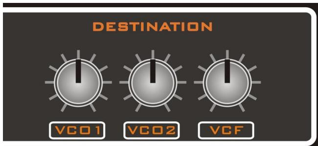
The output CV of the sequencer can be routed to VCO1 pitch, VCO2 pitch and VCF cutoff. The level can be changed using the appropriate control.
