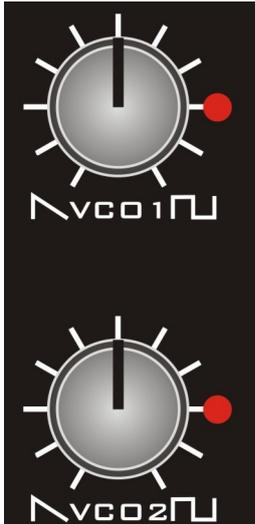
Left; changes the level of VCO1 Sawtooth waveform.
