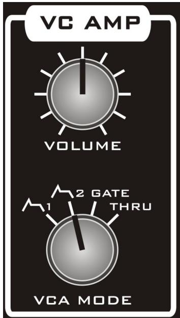
The VCA is an amplifier whose gain can be changed with a modulation signal, typically an envelope.
