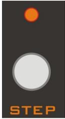
The step button allows you to manually step the sequencer.
