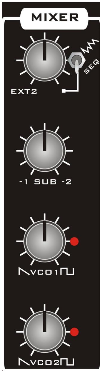
There audio is mixed with the mixer before being fed to the input of the filter.
