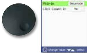
In the example on the side, the „Midi-in“ parameter has been selected. Use the DIAL to change the value currently set for that parameter. Pressing the ESC button takes you back to the main menu window (the changes you have made, now apply). If you want to close the main menu window completely, press the ESC button one more time.
