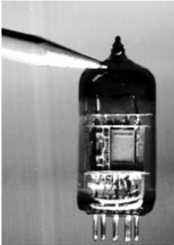
Turn off the amp, and allow the tubes to cool. Now pull out the troublesome tube and replace it with one of the same value (that is, if you're pulling out a 12AX7, replace it with a 12AX7).
