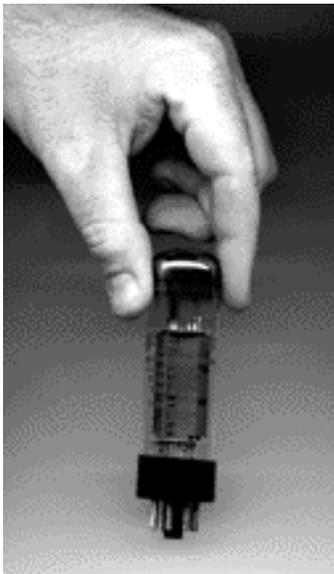
Make sure that the tube is oriented correctly when pulling it out or putting it back in. If you look at the end of the tube and the socket, you'll notice that the nine pins are arranged in an incomplete circle. Always make sure the pins are aligned correctly.
