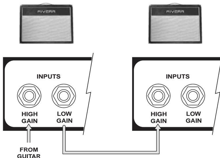
The Preamp and output amp sections, as well as all controls, function normally in this setup. Use a shielded cord. Note: Make sure speaker cabinets are connected to both RIVERA amps.
