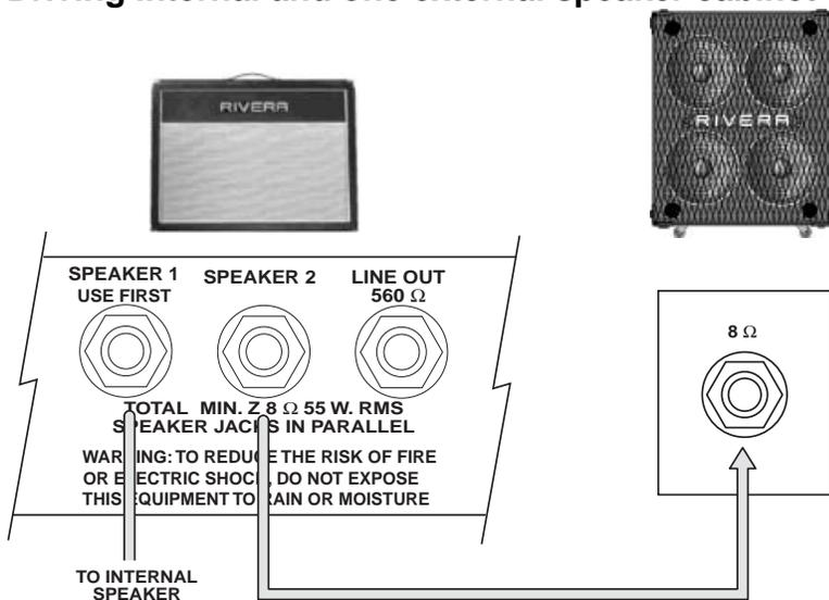
In this configuration, the Quiana is driving the internal speaker load, with an identical impedance external load. Using heavy-gauge speaker cords, connect the output jack labeled Speaker 2 to the speaker inputs on extension cabinets with a minimum 8-ohm impedance and power-handling capacity of 60 watts. Set the Quiana's Impedance Selector to 4 ohms.
